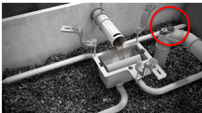
Fig-11: Level probe and alarm box
