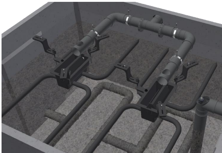
Fig-8 : Split flow device in a 6.5m 3 filter
